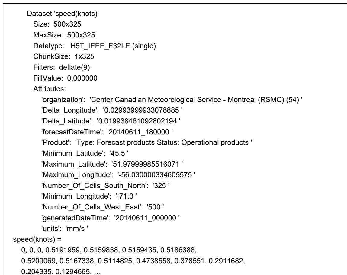
Figure E-3 – A portion of the actual metadata and the gridded current speed data produced by the Canadian Meteorological Service from a model-based forecast. The native format is HDF5
